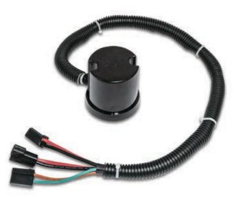
This control provides the switching logic to use low current signal inputs for extending and retracting the actuator rod/screw. It mounts on the back end of Warner Linear's 12VDC B-Track motor/actuator product.
