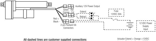
Actuator Extend = Orange +12VDC Actuator Retract = Green +12VDC
